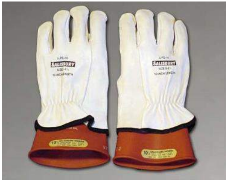
Gloves designed for electrical protection. Note the rubber inserts are rated for a specific level of electrical voltage. Leather outer gloves are designed to protect the rubber inserts. (*2)
