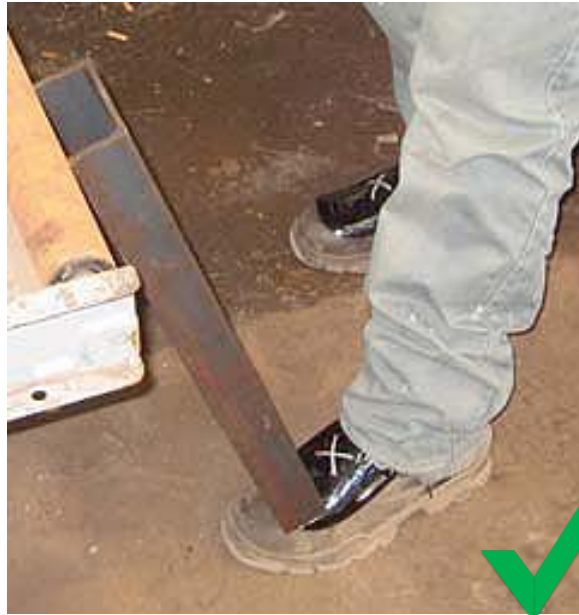
Demonstration of protection provided by the metatarsal guard in this image. (*3)
