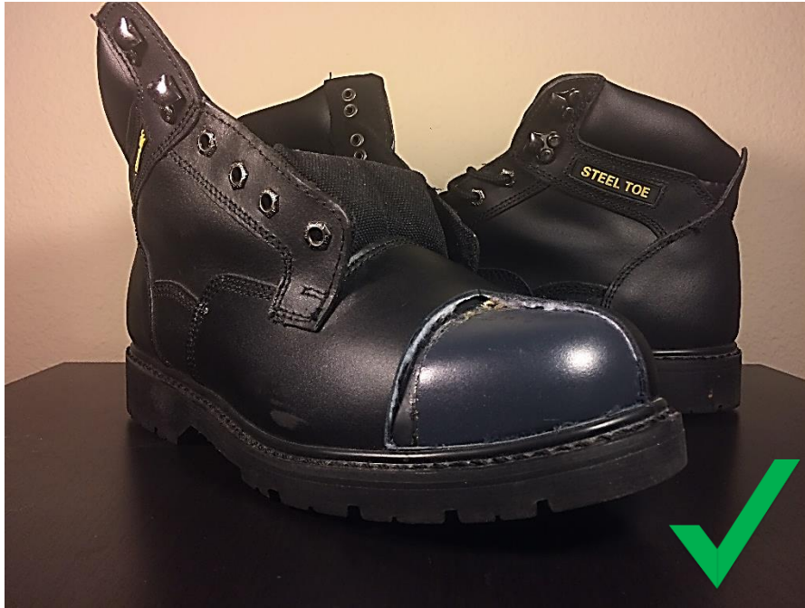
A cut away of this steel toe boot shows the interior steel shell designed to protect the toes of the worker.
